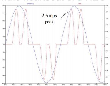
Diode Bridge Rectifiers cause Torque Ripple
