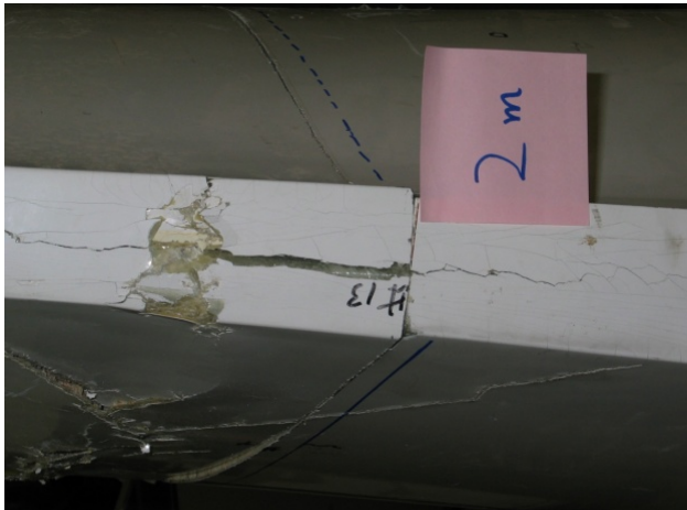
Damage at test peak load of 48.612kN (2 m from root of the blade)
