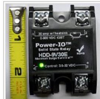
Small IGBT module, rated up to 30 A, up to 900 V
