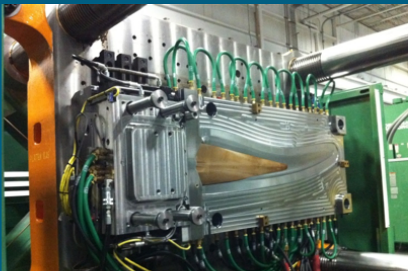
Pika Energy's injection molding tool for manufacturing wind turbine blades. Photo Credit: Pika Energy, NREL 33941
