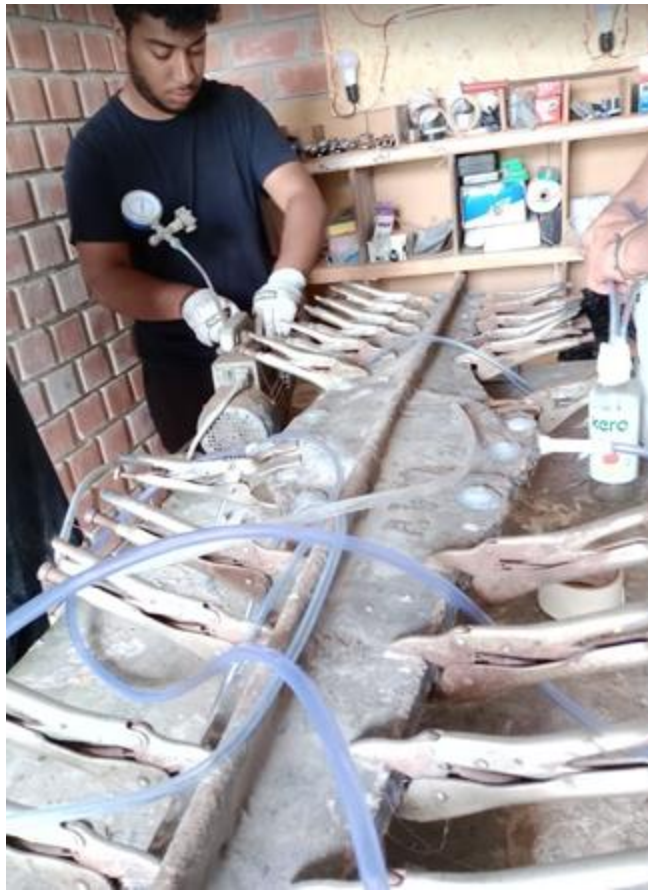
Vacuum Resin Injection Process for Blade
