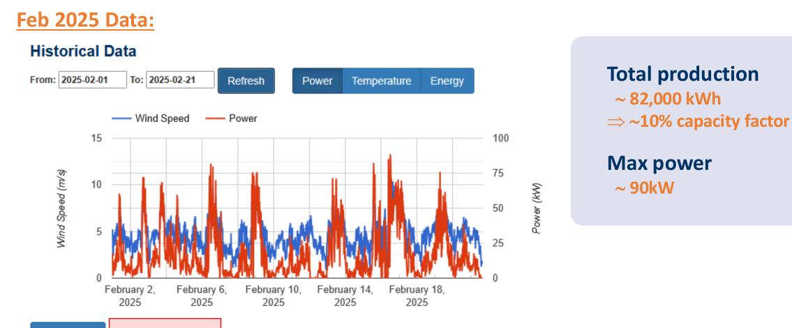
Export CSV Clock Availability: 100% Run hours: 495.3 | Production hours: 495.3 | Fault hours: 0 | Average Wind m/s: 4.7 | Energy Produced kWh: 7,646
